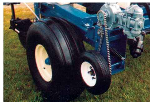
Hydraulic actuated press wheel drive single or twin piston pump. Adjustable drive wheel tension.
