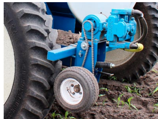
Adjustable Drive tension for positive traction
